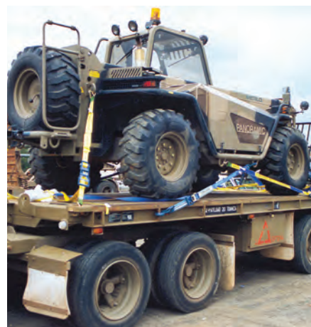
Merlo 4WD forklift combination direct restraint and tie-downs
