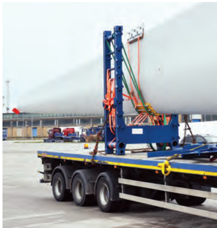
Wind turbine cradle and restraints
