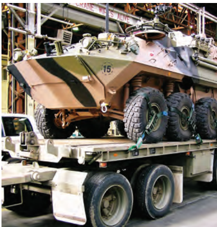
ASLAV 8WD amphibious vehicle wheel restraints
