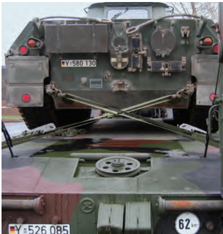
High performance direct lashings for NATO tanks
