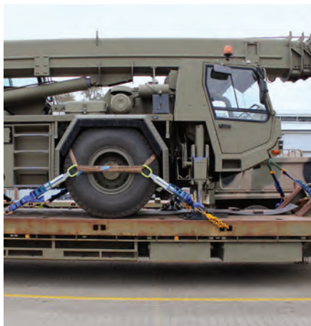
24 tonne Tadano wheel restraints for ADF
