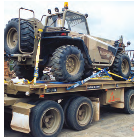
Merlo 4WD forklift combination direct restraint and tie-downs
