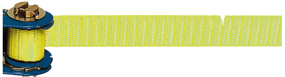
More than 10% cut in webbing
