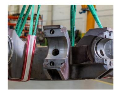
Protect slings from sharp edges, increase work safety and sling service life: secutex-coated protective sleeves are easy to position, dimensionally stable and extremely cut-resistant. **Find out more at www.secutex.com/en**
