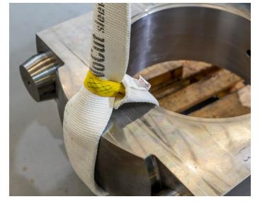
The NoCut<sup>®</sup> sleeve offers optimum cut protection for your textile slings when sharp edges are involved. **Find out more at www.spanset-nocut.de/EN/home.php**
