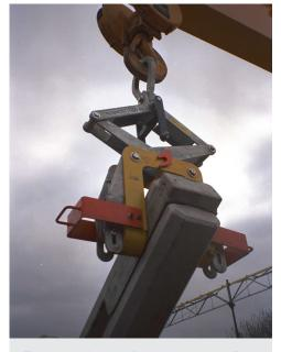
Turning grippers for concrete profiles
