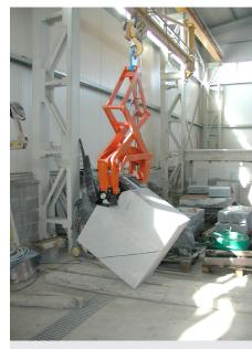
Turning grippers for stone slabs
