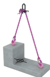
Asymmetrical load Centre of gravity off-centre
