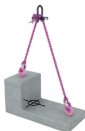
Asymmetrical load Centre of gravity off-centre
