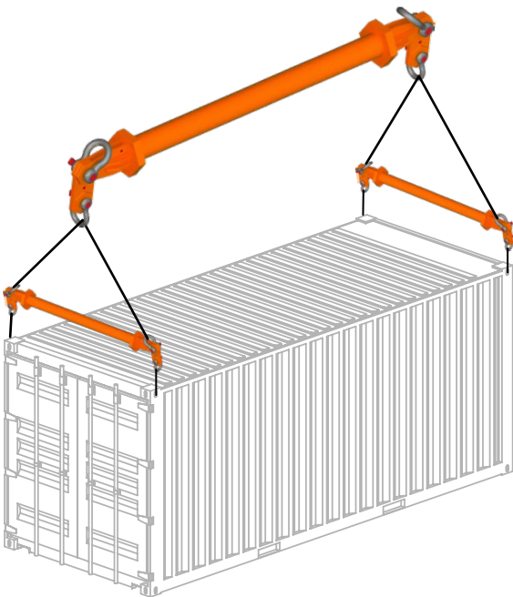
Lifting with vertical twistlocks.
