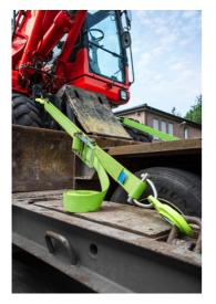
III. 1: The 50mm-heavy duty ratchet lashing system MaXafe shows extremely high tensile strength and low elongation. It is much lighter than a common 75-mm lashing system.
