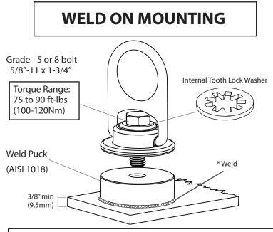
\* Welding procedure must be approved by an engineer or other qualified person to be compatible with any and all structural & operational characteristics of the selected installation location.
