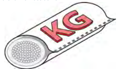
Raised, woven-in load capacity indicator
