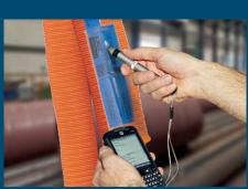
The label of the **Magnum®Plus Flex** is attached to a case that is securely sewn into the protective sleeve. Additionally protected by a foil, all necessary information remains visible at all times.
