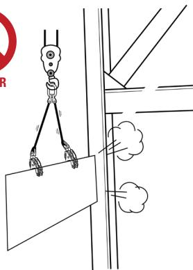
**EN** If a load hits an object the clamp is subject to an impact load which might cause an extra force on the clamp.
