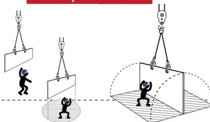
EN **Make sure that the load is lifted from the point of gravity.**
