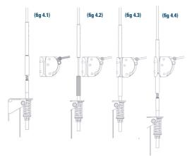
Disconnecting from the lifeline cable must only be performed when in a safe position. The device may be removed from the lifeline at any safe position by performing the direct connection method of gate operation. The device may be removed from the base of the lifeline by operating the base bracket entry gate and sliding the device intermediate bypass slot over the narrow cable.
