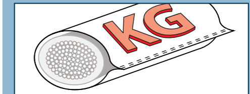
Raised, woven-in load capacity indicator.
