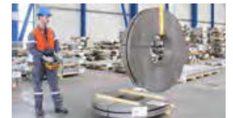
secutex split lifting strap, The solution for secure turning
