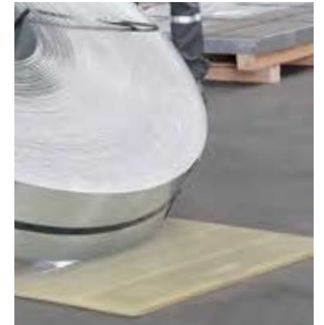
Optional secutex turning mat: no uncontrolled slipping
