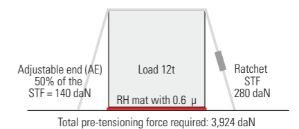
2 t-lashing strap, commercially available, without TFI
