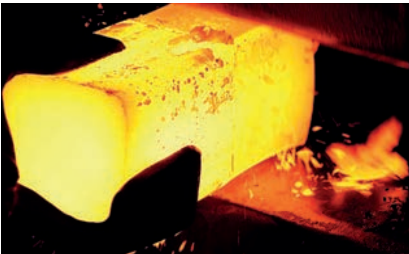
Square billets (edge length 50 to 120 mm) or round bar material (18.5 to 200 mm in diameter) can be used as raw material.
