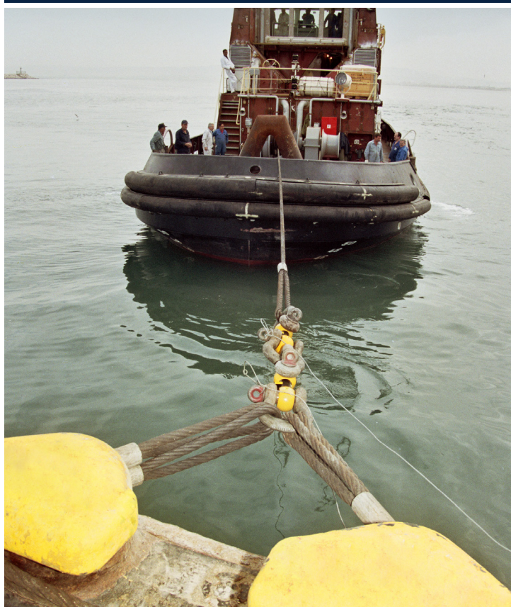
Bollard pull test
