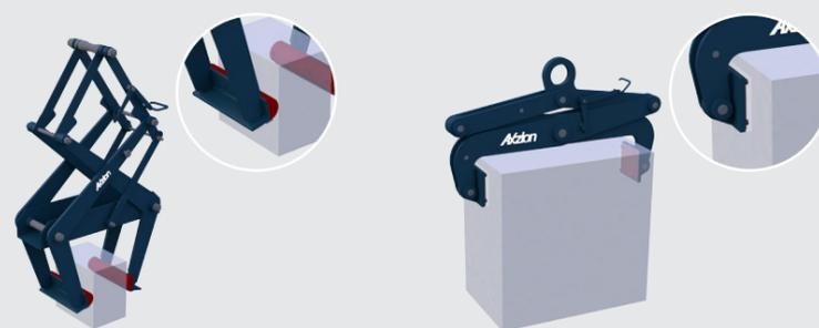
The gripping of the load takes place by frictional engagement. Friction grippers must have a safety factor > 2 against the load slipping out. The coefficient of friction in combination with the surface is relevant.
