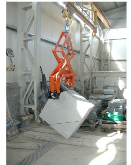
Turning grippers for stone slabs
