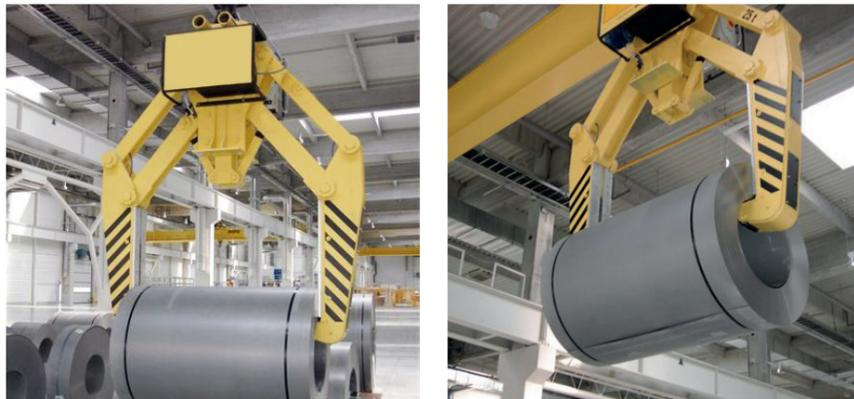
Parallelogram coil gripper
