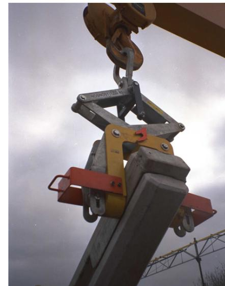
Turning grippers for concrete profiles
