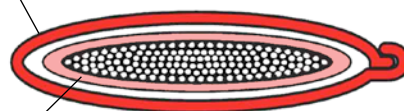
2 The sleeve hose of the Magnum-X smart round sling has a yellow signal colour
