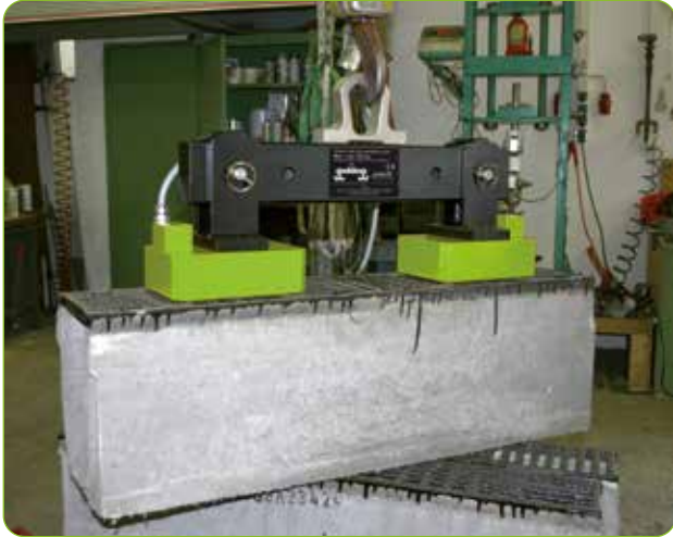
FXE-T Electro-Permanent Deep field Truss
