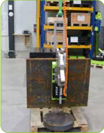
FXE HV device for horizontal/vertical lifting
