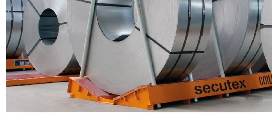
Coilprotect „Altus“, Coil storage in a tall design
