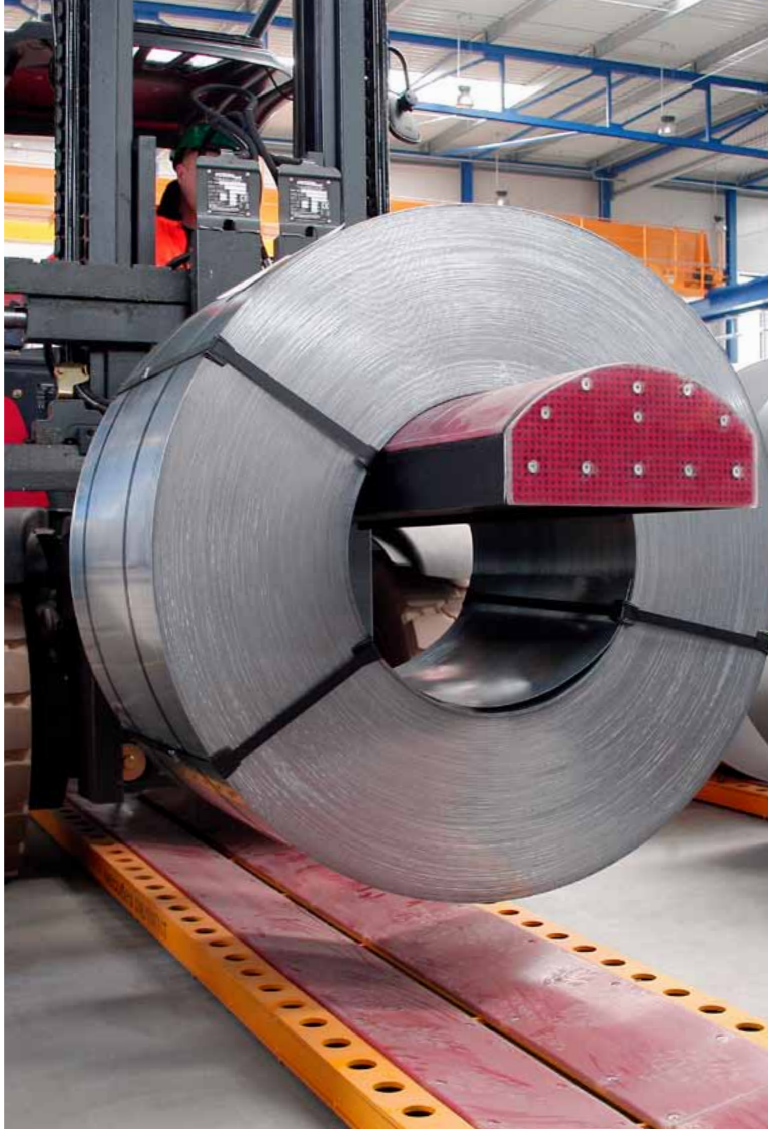
Figure: secutex fork protection - coil without drive-in chamfer.
