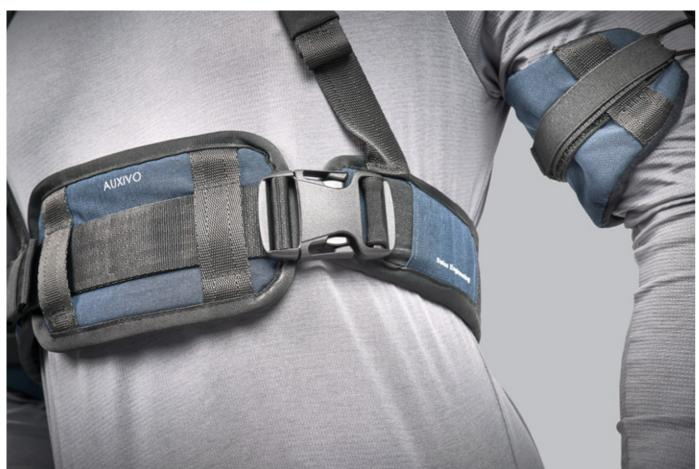
The split-vest design ensures flexible movement and acts as an interface for the mechanical structure, and through the vest, the DeltaSuit is attached to the thorax instead of the hip for unconstrained upper-body movement.
