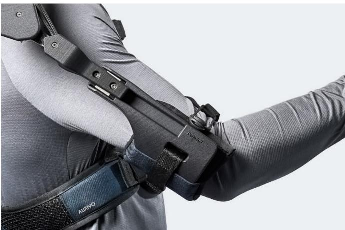
The telescopic mechanism in the arm and elasticity in the split vest ensure maximal anatomical compatibility with the user and a high usability.
