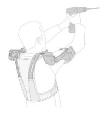
Benefits when manipulating objects While manipulating small objects above shoulder level without a tool, the support provided by the DeltaSuit significantly reduced upper body muscle load. Specifically muscle load in shoulder was reduced by 36%, the neck by 34% and the arm by 37%.
