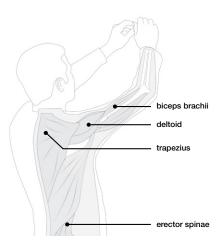
Benefits when using a power tool While fastening screws with a powered drill, using the DeltaSuit significantly reduced muscle load in the shoulder by 33%, muscle load in the neck by 22% and muscle load in the neck by 17%. No significant changes in lower back muscle activity were observed.
