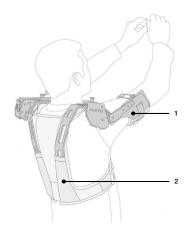
Minimal misalignment and auto-adjustment of size through (1) telescopic arm mechanism and (2) elasticity in the vest
