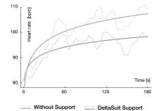
Cardiac cost of fastening screws with a powered drill above the head was 21 bpm. During the study the support of the DeltaSuit reduced the cardiac cost by 15% to 18 bpm.
