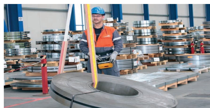
Secumove protective sleeve to help safe lifting and rotating of sharp edged loads
