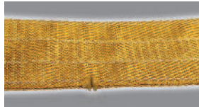
The webbing cross-section is damaged by less than 10 %
